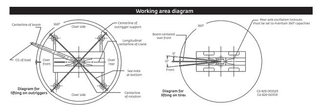
Bold lines determine the limiting position of any load for operation within working areas indicated.
